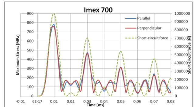
Fig. 8. Maximum Stress for Steel IMEX 700
