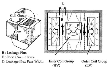
Fig. 2. Short-circuit forces of Shell Type Transformer [11]
