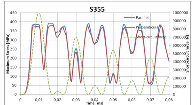
Fig. 7. Maximum Stress for Steel S355
