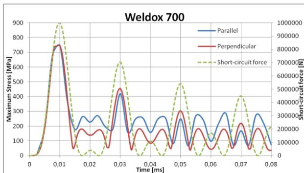
Fig. 9. Maximum Stress for Steel Weldox 700
