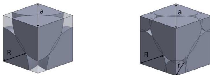
Fig. 1. Compacted structures of fillers in open-cell arrangements, left: uniform-size structure; right: dual-size structure (Kou et al., 2008)
