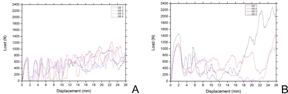
Fig.4.Compression tests results– Uniform-Size Structure (A); Dual-Size Structure (B).
