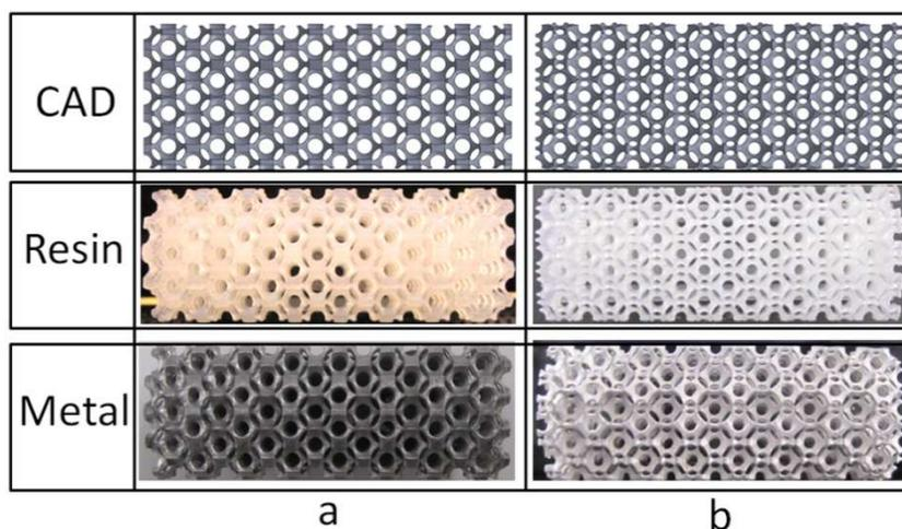
Fig. 2. CAD, resin and metal specimens obtained: US cellular structure (a) and DS cellular structure (b)
