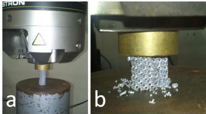
Fig.3. Compressive tests: (a) initial stage; (b) final stage.
